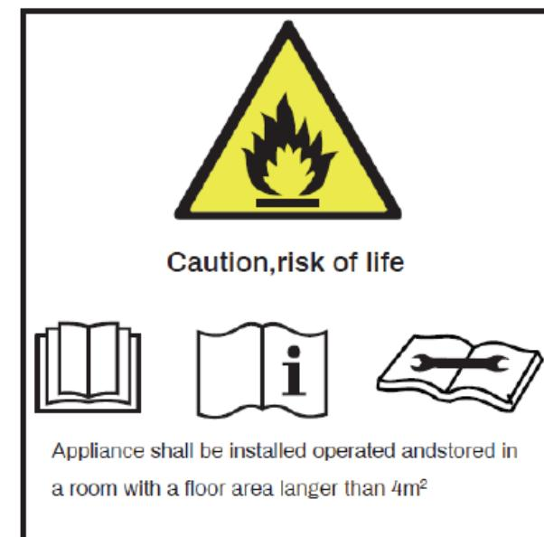
Appliance shall be installed operated and stored in a room with a floor area larger than 4m<sup>2</sup>
