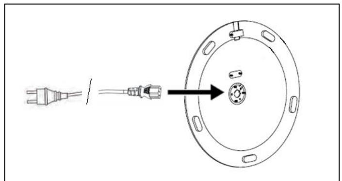
**Step 5:** Connect the female plug to the plug connector of the heating cap. Secure this connector using the clamp included in the package. Make sure that the arrow of the clamp is directed towards the top of the patio heater.
