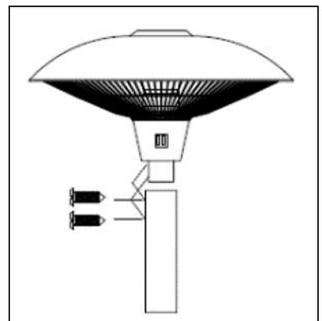
**Step 7:** Check whether the telescopic tube is extended to the maximum. Secure the telescopic tube in this maximum position by tightening the black coupling nut.
