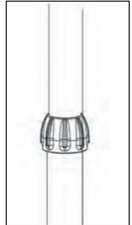
**Step 4:** Lead the female plug of the mains lead through the base and the bottom, centre and top tube.
