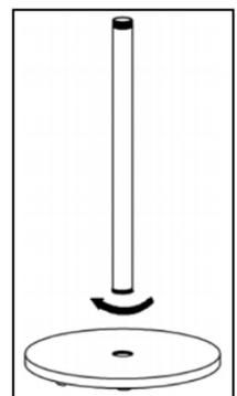
**Step 2:** Attach the top (telescopic) tube onto the bottom tube by screwing them to each other.
