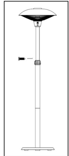
**Step 8:** You can now adjust the height by slightly loosening the coupling nut and slightly pulling or lowering the top tube. Subsequently, retighten the coupling nut at the required height.
