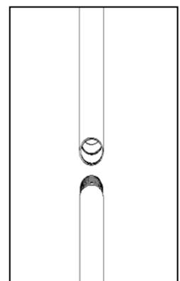
**Step 3:** Pull the inner (telescopic) tube out of the outer tube and secure it by tightening the black coupling nut.
