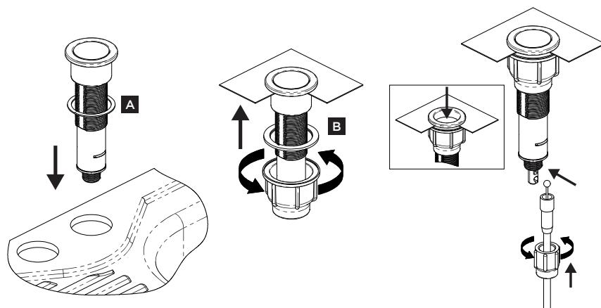
Adjust the stainless steel drain to the optimum position by the screw.
