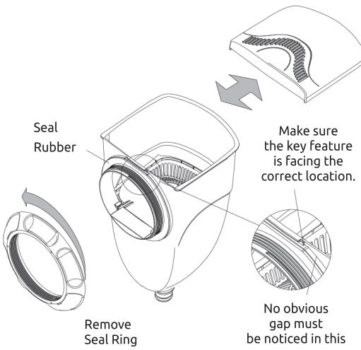
**2.** After placing the threaded intake of the skimmer inside its corresponding pool hole, screw back the seal ring tightly on its place.
